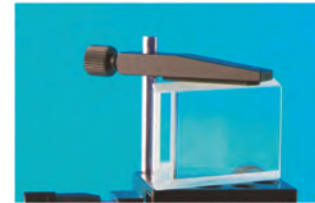
Optics is held by rubber padded clamp
