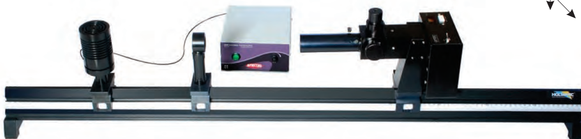
Fig. Experimental setup for determination of the temperature of an artificial star by photometry.
