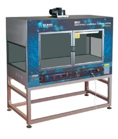
HOLMARC's HO-FH-06 model fume hood provides an enclosed atmosphere for electrospinning. An enclosed chamber is necessary to protect the user from pollutant air caused by solvent evaporation during the process. It comes with an exhaust fan attached or optionally with a duct of custom dimension so that it can be connected to an exhaust duct available onsite.
